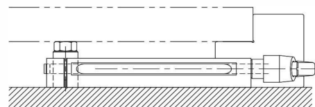
Low profile allows reaching far underneath low workpieces.
